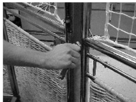
f.) When both independent door locks are in position, the central over-lock can be rotated into position.
