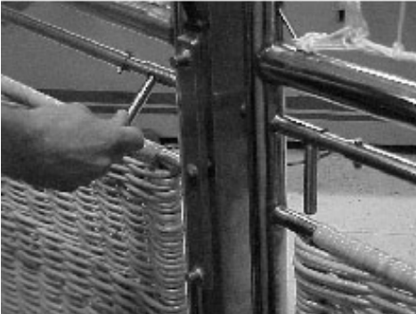
e.) Both doors are to be fully locked.
