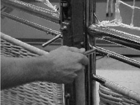
c.) The locking lever slides across horizontally until the bolt is fully into its locating hole.
