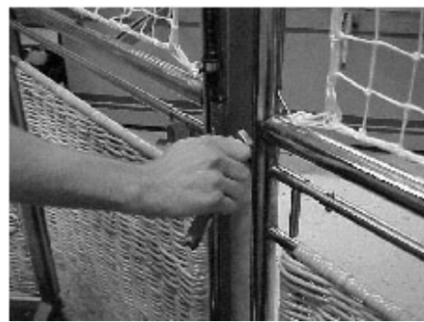
f.) When both independent door locks are in position, the central over-lock can be rotated into position.
